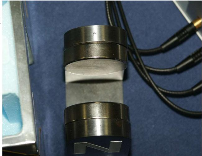
With a special 2-temperature stage and our sampleholder the Hall system using this magnet is an easy and nonexpensive system for quick and reliable van der Pauw and Hall measurements.
